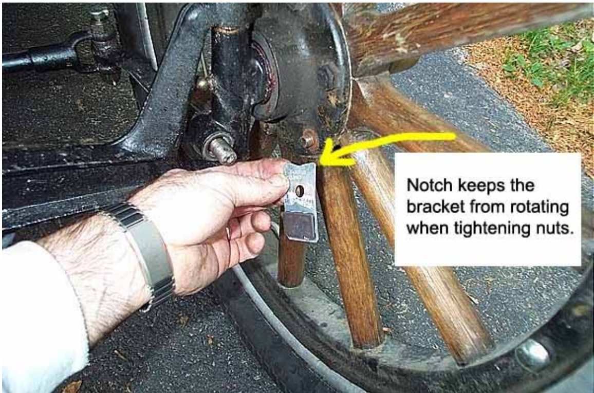
Figure 3 – Attaching Finished Bracket to Front Hub
