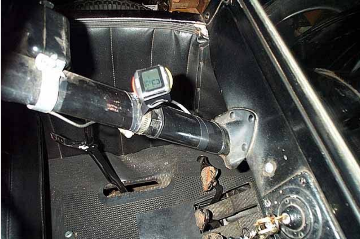
Figure 11 – Finished Installed Speedometer
