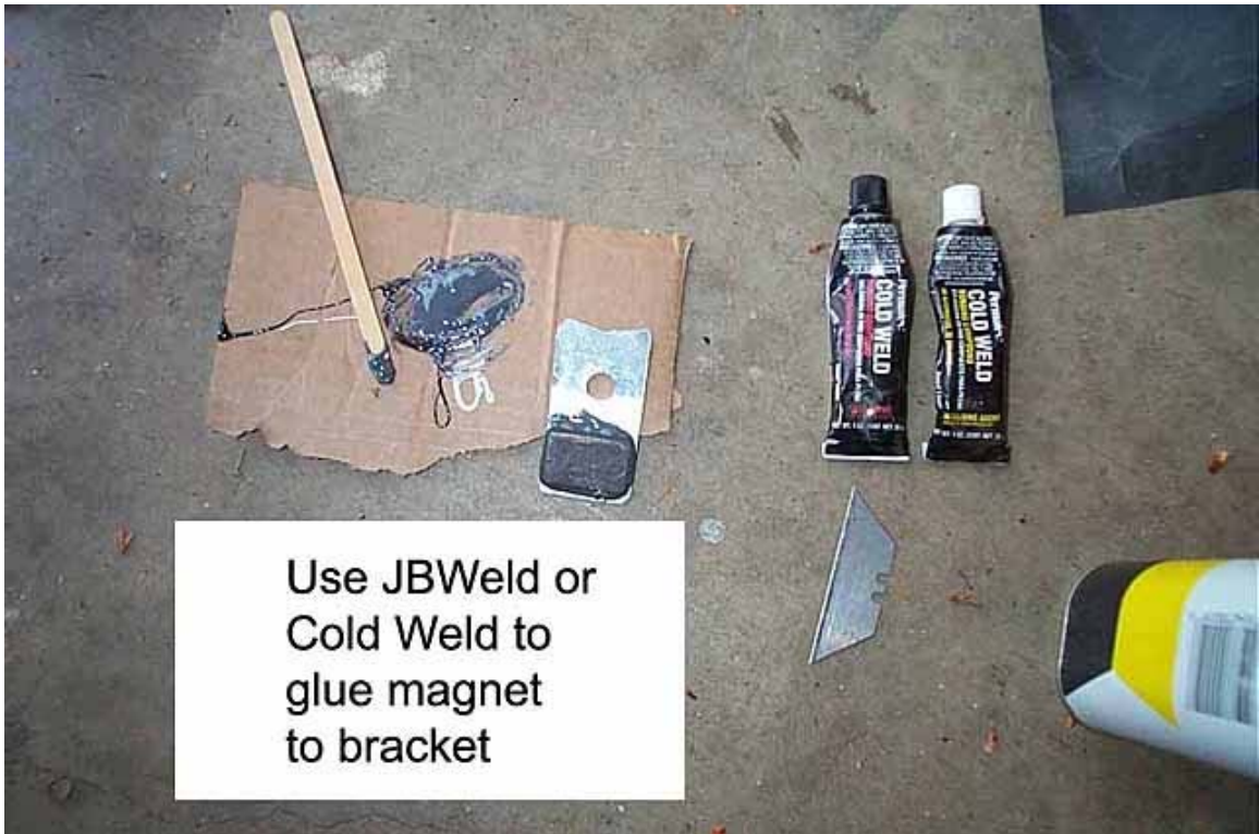
Figure 2 – Epoxy Magnet to Bracket
