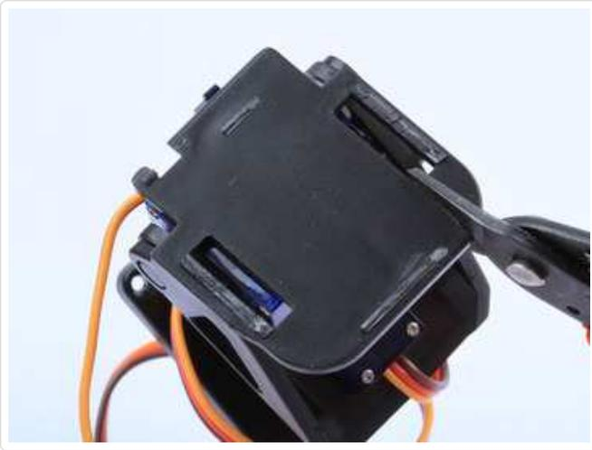
the back of the camera module. Two cuts, as shown in the photos will remove the top left side of the bracket.
