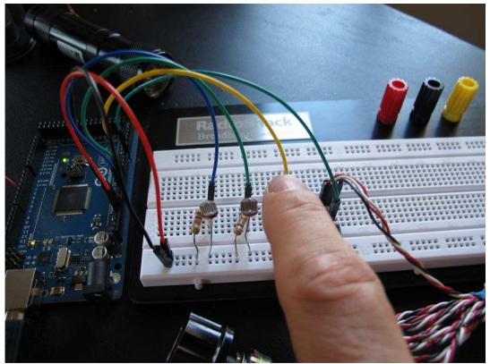
stop. Move your finger from sensor to sensor. You should hear a series of notes (a different note for each sensor).
