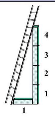
Place the base of non-self supporting ladders out away from the wall or edge of the upper level one foot for every four feet of vertical height (1:4).
