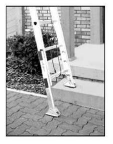
Use a wood or plastic wedge or a ladder leveler leg when using ladders on unven surfaces.
