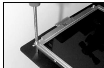
**FIGURE 4.2 Removing the front surround and the display unit from the mounting plate pillars on the Multitrend V5**
