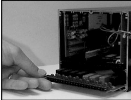
FIGURE 2.2 Inserting the Alarm card
