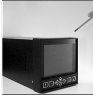
**FIGURE 3.1** Removing the front panel
