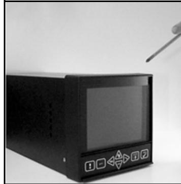
FIGURE 7.2 Removing the front panel
