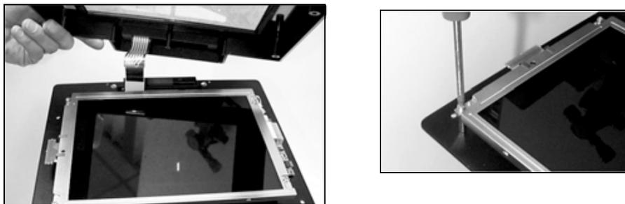
**FIGURE 6.4 Removing the front surround and the display unit from the mounting plate pillars on the Multitrend Plus**
