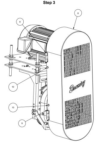
1.8 Using the hinge pins provided (Item 9), attach the guard front (Item 8) to the guard back.
