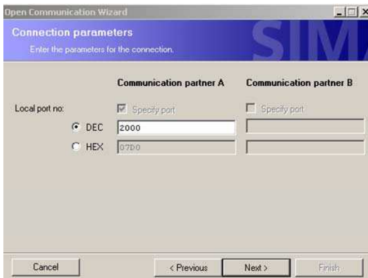
Figure 5-7 ports of the TCP connections
