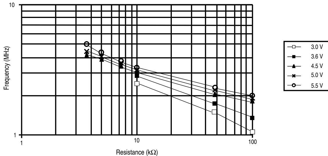
Figure 1. Typical Internal Operating Frequency at 25 °C for High-Speed RC Oscillator Option
