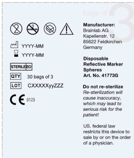
Figure 2: Example of label on the side of the Brainlab dispenser box Art.No.41773G (containing 30 packs of Art.No. 41772G)
