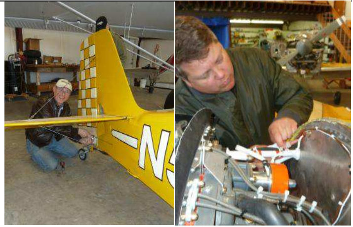
(left) Paul Dye tends to the tail wheel assembly (right) Michael Stephan plugs some baffling holes
