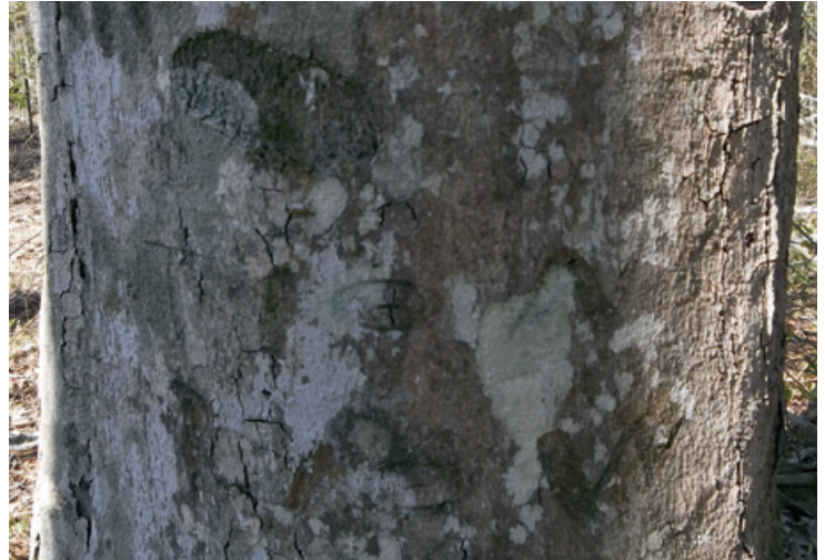
Picture of a witness tree found on a GLO corner. This beech was marked by a U.S. deputy surveyor in 1843, and is still standing today.
