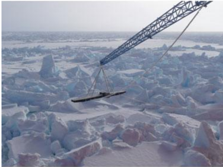
Figure 10. An electromagnetic induction device for measuring sea ice thickness, called the "Worbot" after Australian sea ice scientist Tony Worby, mounted on the icebreaker Aurora Australis . (K. M. Golden)
