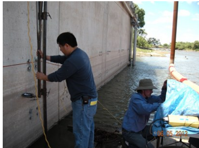
Helping perform a hydraulic velocity evaluation of fish screens on the San Joaquin River for the Patterson Irrigation District
