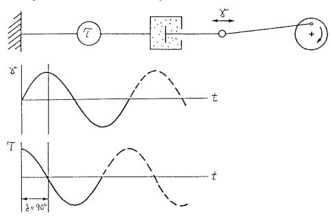
The stress of a purely viscous material depends on the deformation velocity. At the two maximum strain values, the strain velocity is zero, because the system changes direction. Therefore we find that stress and strain are  $90^{\circ}$ out of the phase ( $\delta=90^{\circ}$ )
