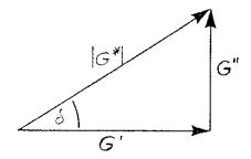
The absolute magnitude of the complex modulus G\* can now be calculated as the peak stress divided by the peak strain:
