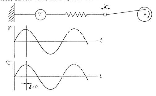
The stress of an ideal elastic material depends on the degree of deformation. Therefore we find that stress and strain are "in-phase". There is no phase shift (  $\delta$  = 0°).
