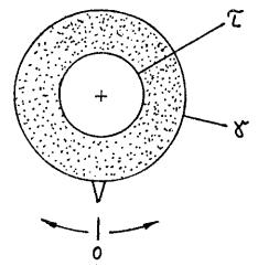
With this coaxial cylinder system we generate an oscillating deformation with the outer cylinder and measure the torque response with the inner cylinder.
