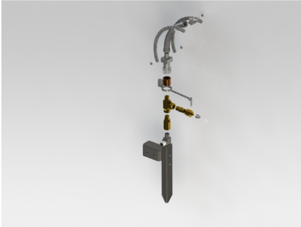
Figure 4 - Exploded view of sprinkler assembly
