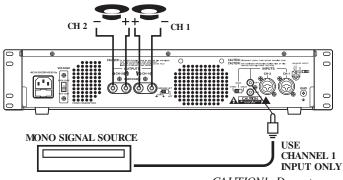
CAUTION! Do not use balanced and unbalanced inputs simultaneously!!
