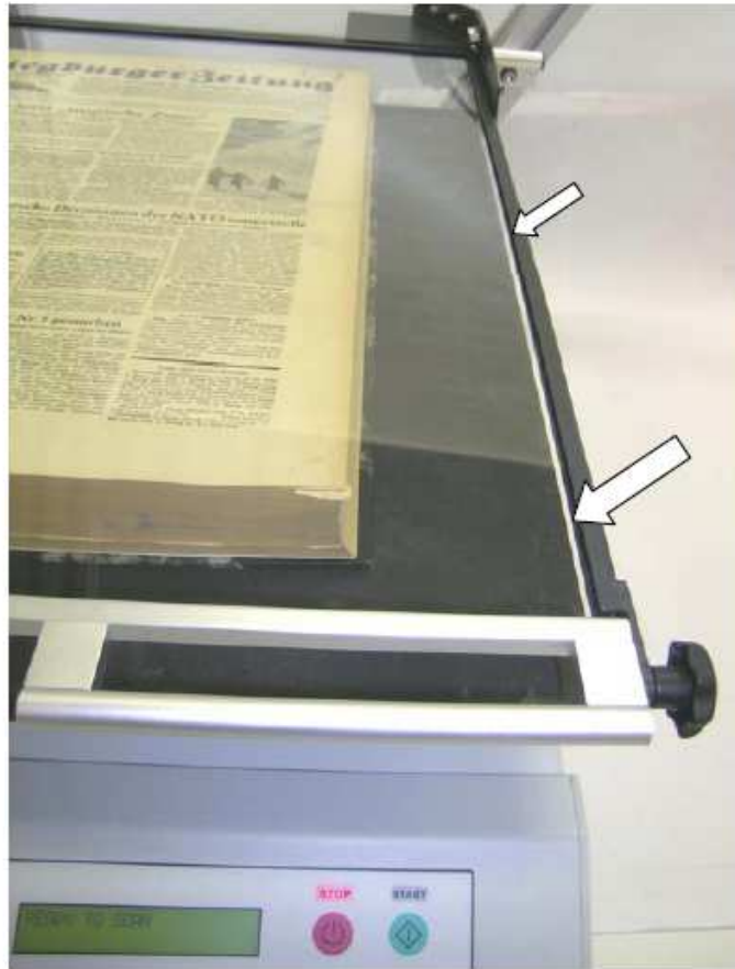
Picture 8: Horizontal alignment check
