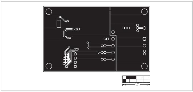
Figure 6. MAX5217 EV Kit PCB Layout—Solder Side
