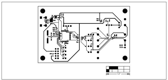
Figure 5. MAX5217 EV Kit PCB Layout—Component Side
