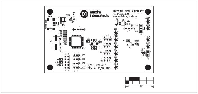
Figure 4. MAX5217 EV Kit Component Placement Guide—Component Side
