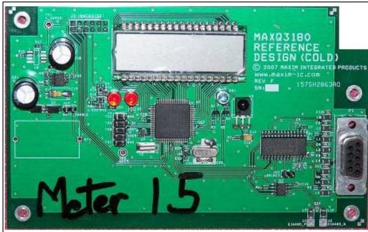
Figure 11. The cold board of the reference design.
