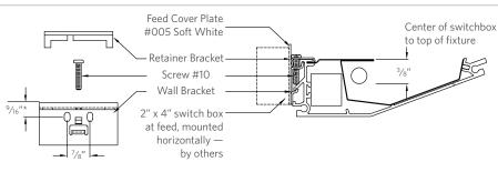
\*Dimension shown is from mounting hole to top of luminaire
