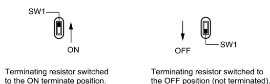
Figure 4-9 Switch Positions for Bus Terminating Resistors
