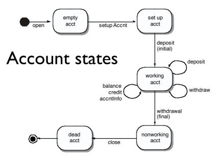
Here's an example of a finite state machine representing an Account class going through a number of states. Transition coverage means testing each Account method once. (From Pressman, "Software Engineering – a practitioner's approach", Chapter 14)
