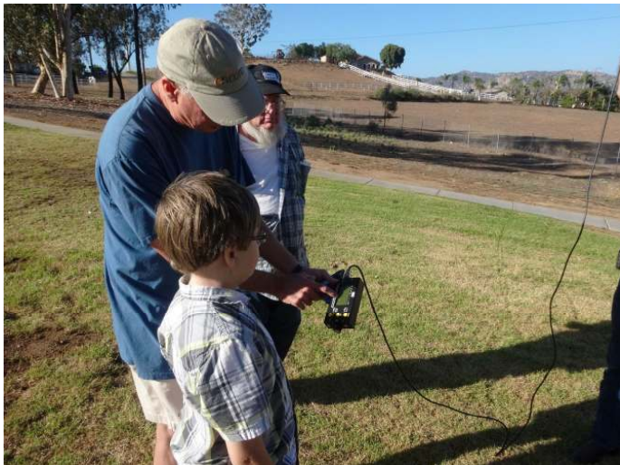
Mike KF6SJ shows Nevan how to use an antenna analyzer to check out the complete antenna.
