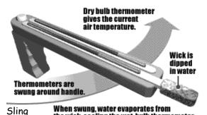
Sling When swung, water evaporates from the wick, cooling the wet-hulh thermometer. Psychrometer Dryer air results in lower temperature.
