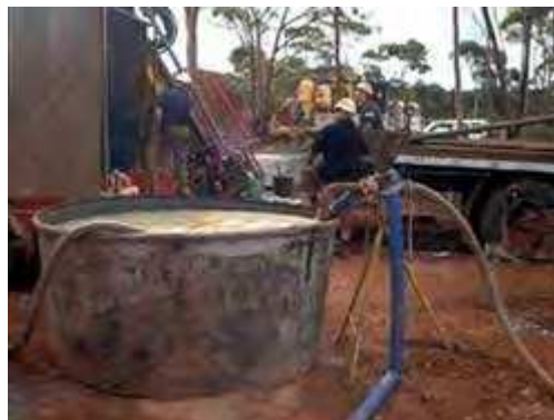
Fig.2 The photograph shows drilling mud being mixed ready to use
