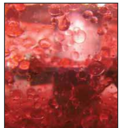
Dispersion of droplets in a liquid-liquid-extraction column
