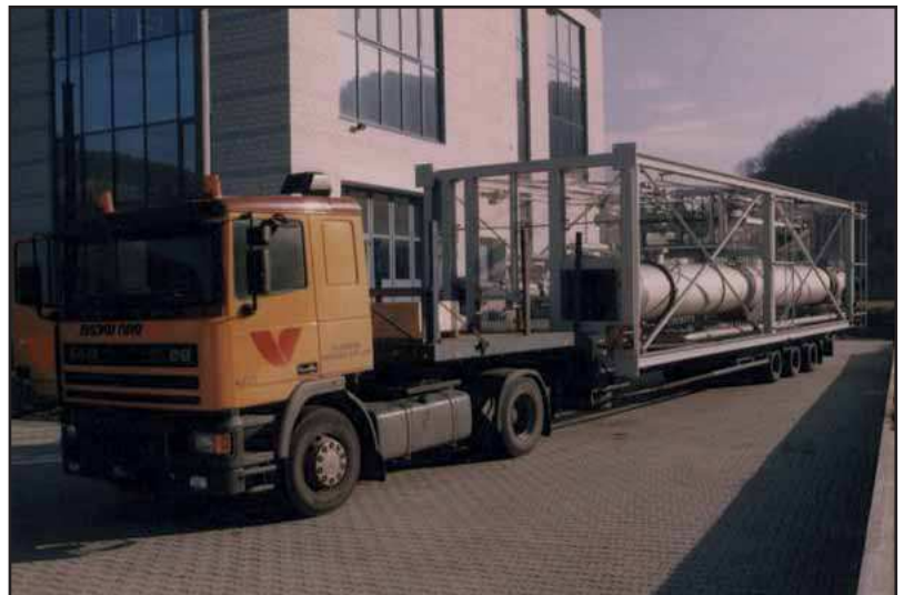
Transport of a pre-assembled skid-unit
