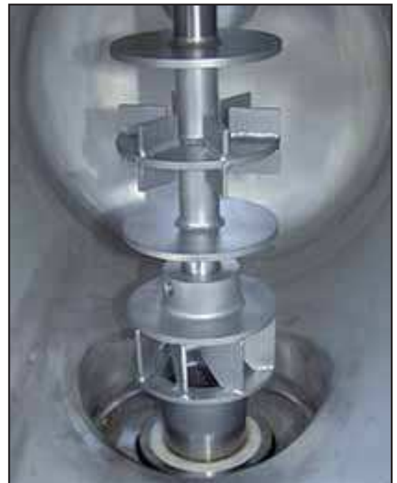
Pump-mix-turbine from mixer-settler type MST 300
