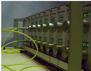
Figure 1. JDSU SWS Test Station for DWDM Component and Module Measurements
