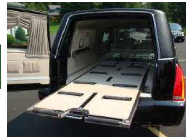
HEARSE S&S "Victoria" professional hearse with extended table easing the pall bearers duty
