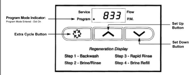
1. The first option setting display that appears in the Program Mode is Treated Water Capacity. Using the Set Up or Down Buttons, set the amount of treated water that can flow through the unit before a regeneration is required. For Example:
