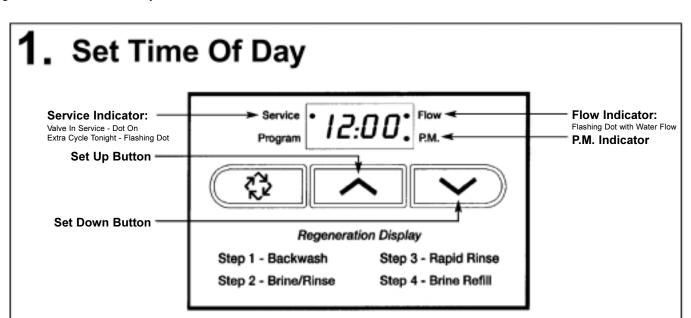
Push either the Up or Down Set Button once to adjust Time of Day Display by one digit. Push and hold either Up or Down Set Button to adjust Time of Day Display by several digits.
