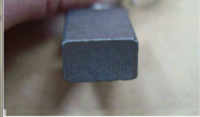
Illustration: Normal brush wear on a good brush
