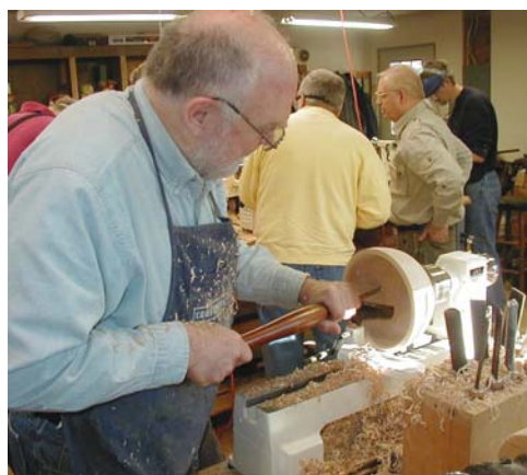
David Winter cleaned up the interior finish of his bowl with his favorite 1/2" thick scraper.
