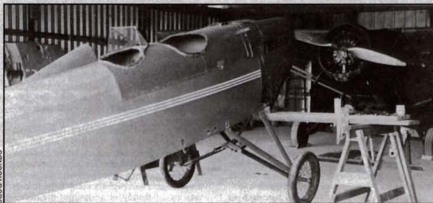
This Travel Air 2000 belongs to Doug Rounds of Zebulon, Georgia. The aircraft was found in the condition shown in this picture. It last flew in 1939. It was re-covered in 1955 but was not completed and flown. Fabric still checks at 70 pounds plus. There are only 1,100 hours on the airframe, and it is strictly stock—it has never been an ag plane. Doug has all the papers, which reveal the 2000 flew mail in Nebraska and Iowa. He also has an old bill of sale signed by Walter Beech and notarized by Olive Ann Mellor—later Walter's wife.
