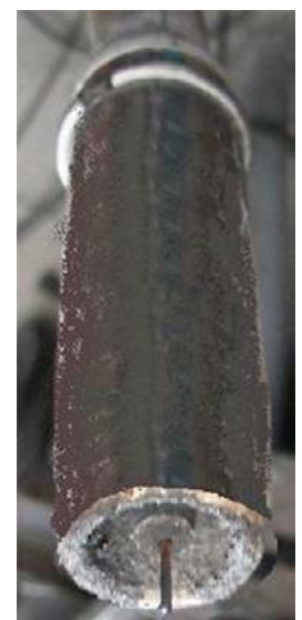
Fig.17. Nozzle and contact tube after MIG welding (5 min), without the protective coating; visible spatters.
