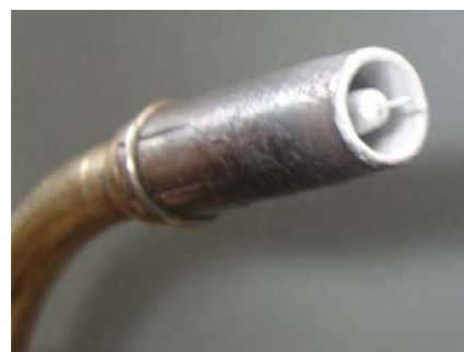
Fig. 1. MAG welding torch tube with anti-spatter substance coating
