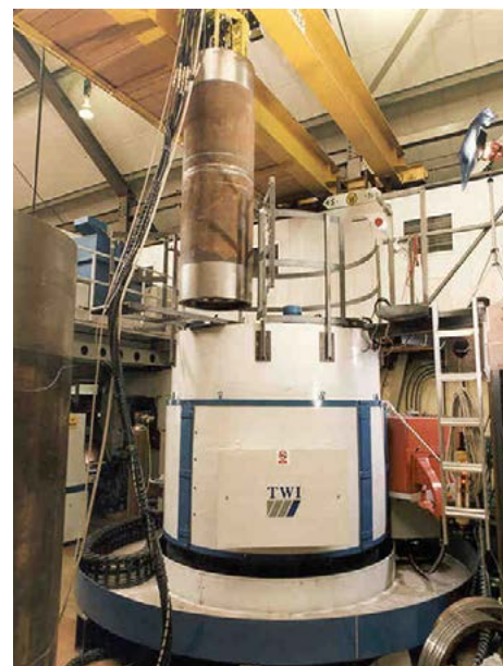
Fig. 9. Example of a specialist electron beam welding machine for welding subsea pipelines [10]
