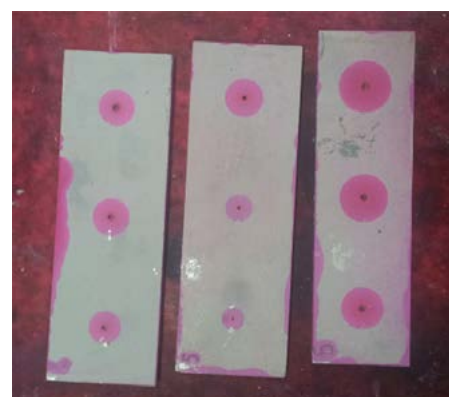
Fig. 4. Samples with developed indications of simulated pores.
