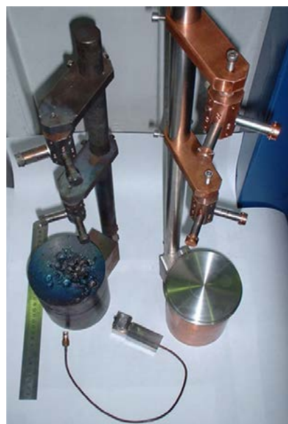
Fig. 18. Electron beam quality control device Probe Beam by CVE [13]
