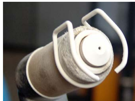
Fig. 22. Plasma nozzle, casing and guide with anti-spatter substance applied; view before plasma cutting
