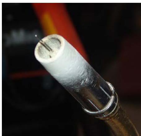
Fig. 19. Nozzle and contact tube with the anti-spatter substance applied, after MIG welding (5 min).
