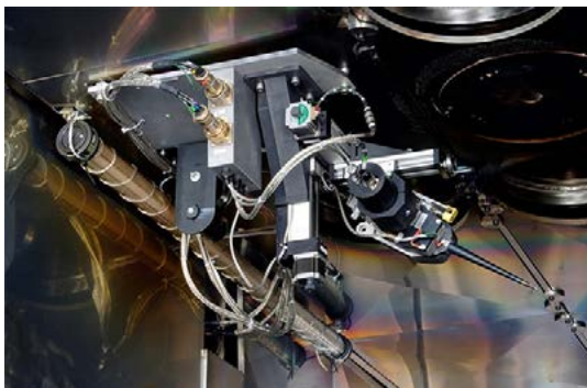
Fig. 15. Electron beam welding electrode wire feeding system [4]
