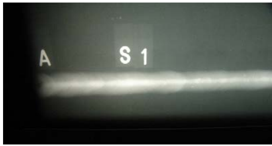
Fig. 6. Radiogram of the weld made with the excessive amount of anti-spatter substance in the weld groove, quality level B according to PN-EN ISO 5817
