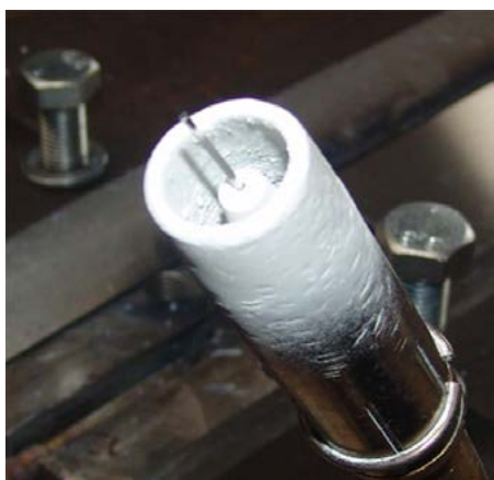
Fig. 18. Nozzle and contact tube with the anti-spatter substance applied; view before welding
