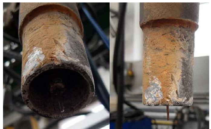
Fig. 16. Nozzle and contact tube coated with the anti-spatter substance, after MAG overlay welding (10 min).
