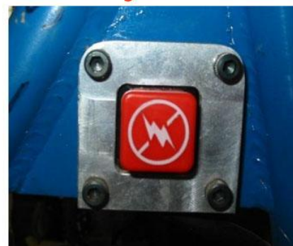
The machined block constraining the switch
