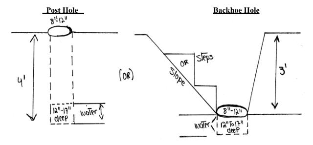
A posthole digger, auger or backhoe can be used to dig the percolation test holes. If a back hoe is used, dig the backhoe hole 3 feet deep, with 2 steps or a ramp. Put a test hole 1-foot deep and 8 to 12 inches in diameter in the bottom. Installation of absorption areas (i.e. drywells) deeper than three 3 feet require the permission of the Environmental Health Department. All dry wells shall be designed by an Engineer registered in the State of Colorado.
