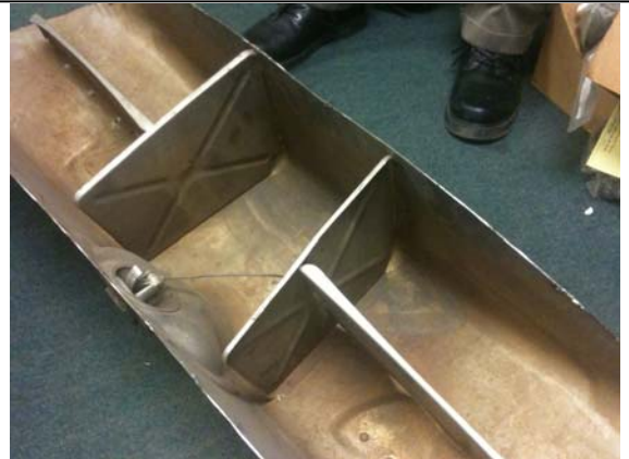
Also at the technical meet was a Model A gas tank with the top panel cut off, something club members don't ordinarily see. The shapes of the sheet-metal baffles in the tank vary from year to year but are similar to this one in the photo.
