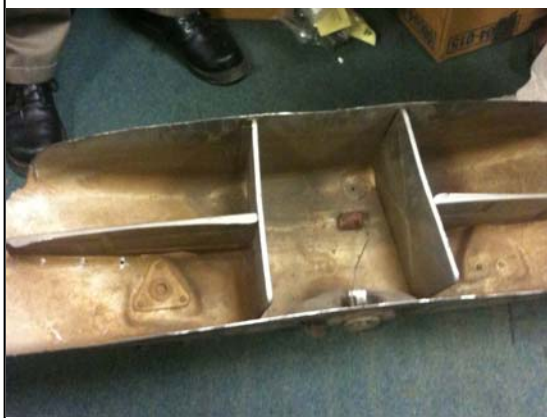
Also at the technical meet was a Model A gas tank with the top panel cut off, something club members don't ordinarily see. The shapes of the sheet-metal baffles in the tank vary from year to year but are similar to this one in the photo.
