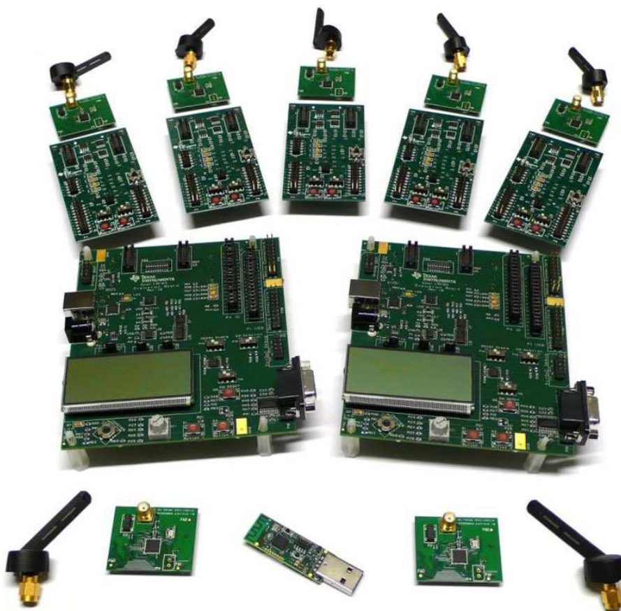
Figure 1: CC2530ZDK – Hardware Included in the CC2530 ZigBee Development Kit
