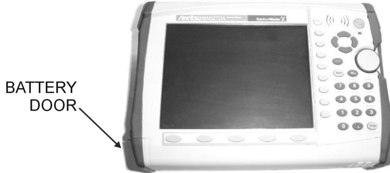
Figure 7. Battery Access Door Location
