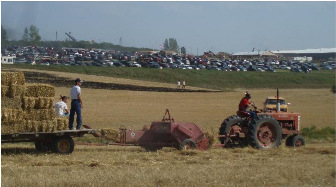
19) IH 12' 120 (do I have that correct?) windrower powered by a Farmall M. Case pull type combine in the background powered by Wisconsin and pulled by an Oliver OC 3.
