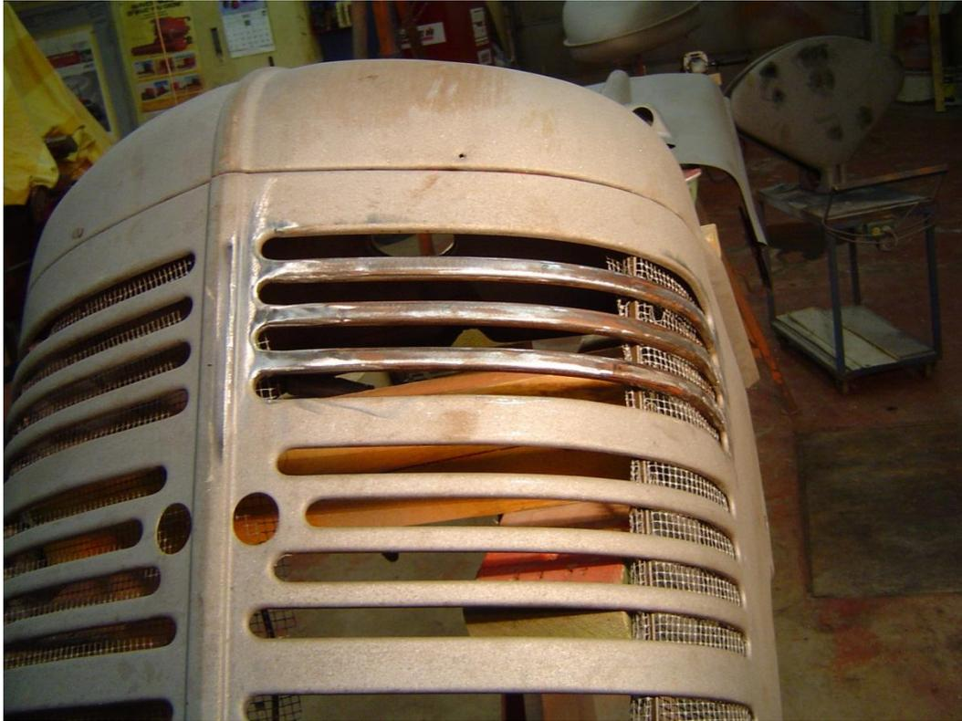
Once they were welded and the welds cleaned up the assembly is coated with a couple coats of 2k high solids primer. I like high build primer because it fills in almost any kind of pitting that you can think of. I like to block sand it with 320 wet paper (no dust). Just remember the better you sand, the flatter the paint will lay out.
