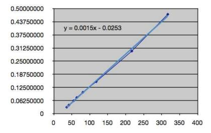
So, once the laser is shined onto the target object and the pfc value of the laser spot is received, an angle  $\theta$  can be calculated using the slope-intercept equation and passed to the trigonometric function to determine the actual distance the range finder is from the target object.
