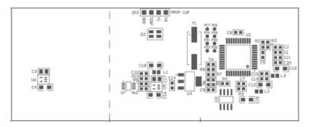
A Prop Clip (Parallax #32200) or Prop Plug (Parallax #32201) can attach to the four pads (JP2) on the back of the LRF for reprogramming of the Propeller's firmware.
