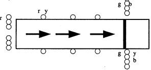
Alternate marking: clearly visible to pilot, not misleading, secured in place, material which will not damage aircraft.
