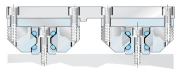
The master fixed rail should always be established straight and true first, within the maximum straightness deviation specified in paragraph 9. With parallel rail arrangements, both rails should be mounted on the same mounting surface elevation and treated with equal surface preparation and tolerancing practices. Precise alignment in terms of spacing, parallelism and height is very important.
