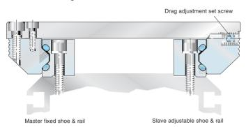
Aluminum roller guides consisting of single sided rails and roller shoes can be varied in rail spacing. They are well suited for assembly on structural aluminum extrusions, due to their homogeneous corrosion resistance and temperature behavior.
