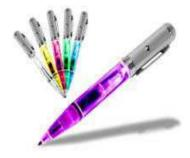
Light pen is a pointing device which is similar to a pen. It is used to select a displayed menu item or draw pictures on the monitor screen. It consists of a photocell and an optical system placed in a small tube.
