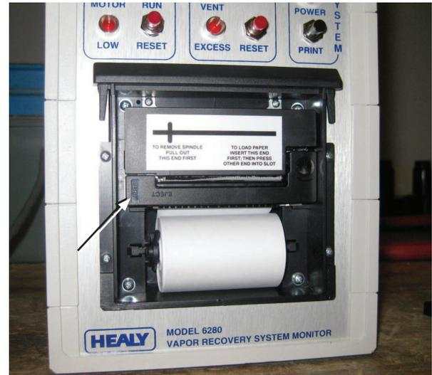
**Figure 13: Remove Printer Ribbon Cartridge**
