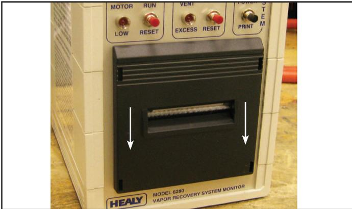
**Figure 11: Remove Printer Cover**
