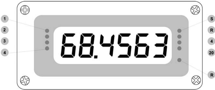
Figure 25. Front Panel LED Indicator Locations
