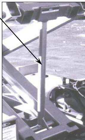
Maintenance lock properly engaged
