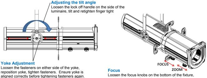
Loosen the focus knobs on the bottom of the fixtu gently slide lenses forward or backward for focus and zoom, tighten focus knob once focused.
