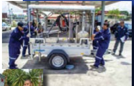
TEAMWORK: Inspectors of the Legal Metrology Inspectorate (LMI), TTBS, prepare the calibrated MVU for verification of fuel dispensers.
