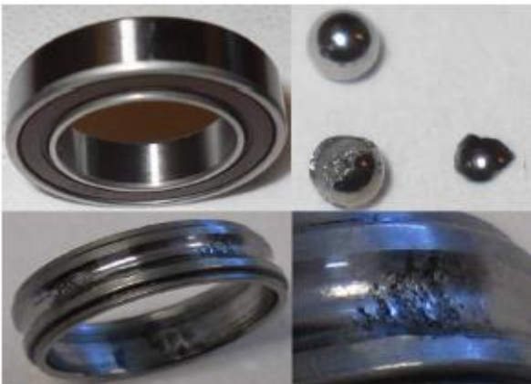
Fig. 4 Normal and degraded bearings
