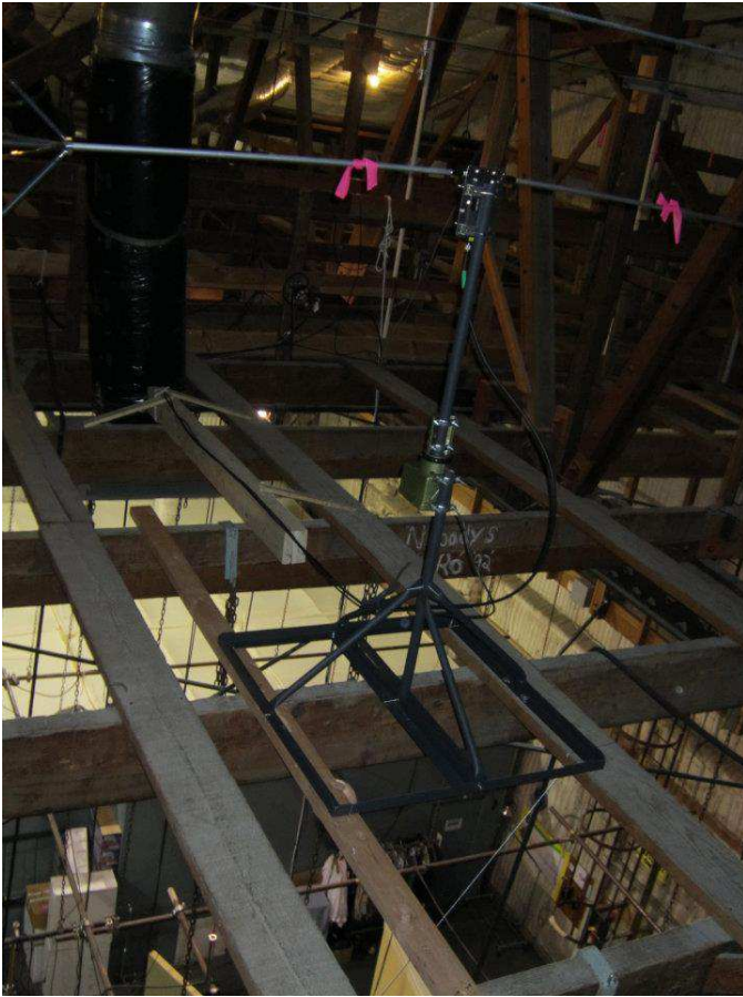
A Comet CHV-5X (multiband rotatable dipole) mounted 50 feet above Mike's office set.
